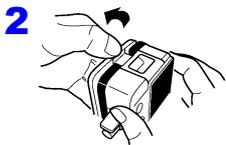
**2** Hold the battery cover while separating it from the logger
