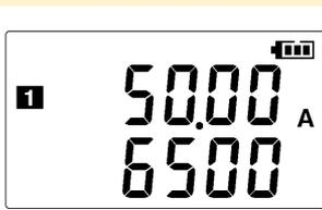
**1** Press the **SET** button to display the CH1 range setting.
