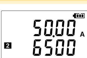
**2** Press the **(+)** and **(-)** buttons to select the clamp sensor model and measurement range.
