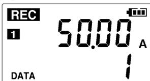
**14** Press **(+)** and **(-)** on the logger to confirm that the recording count is incrementing, and that recording data (maximum and minimum values) are displayed.
